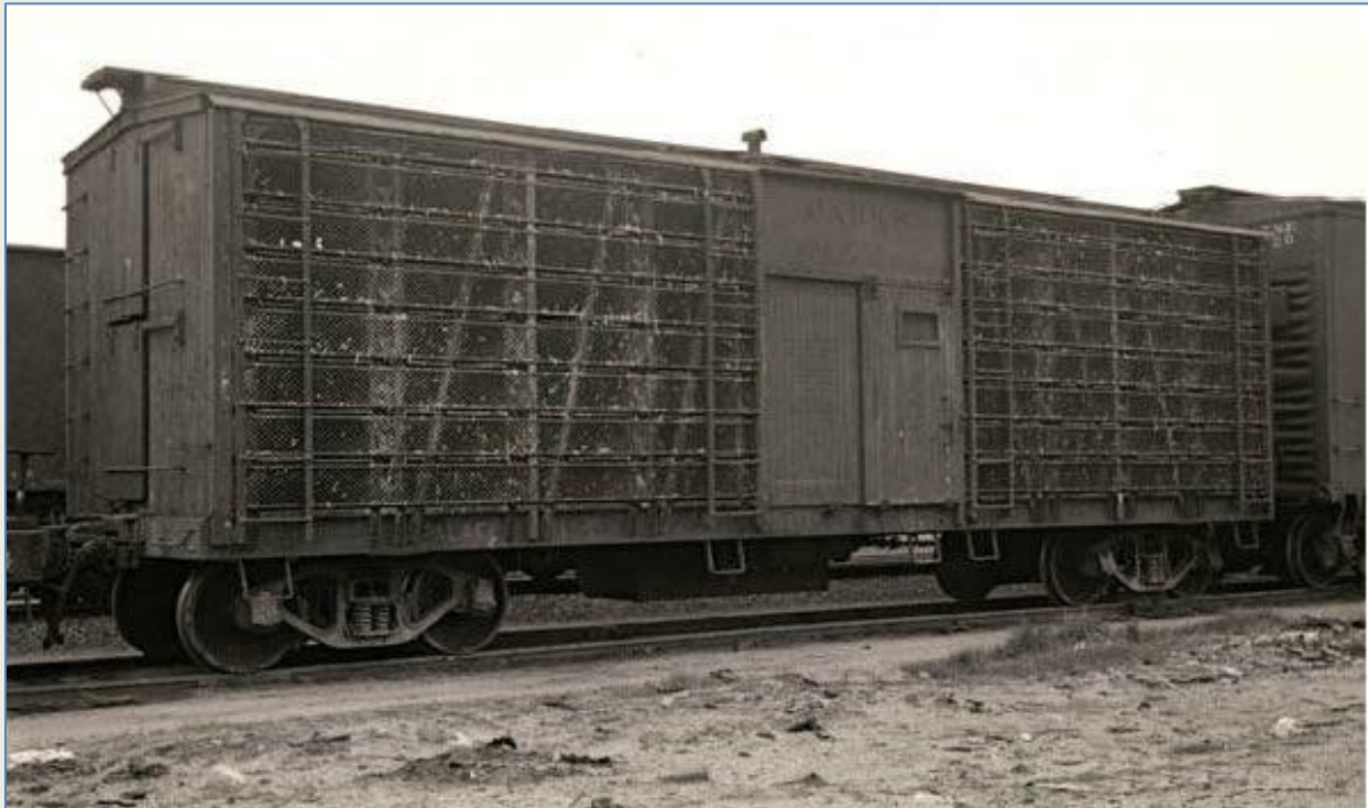
Sometimes called "cackle cars" for obvious reasons, live poultry cars were undoubtedly noisy and smelly places. Just imagine if you were the carman or attendant who had to live with 5,000 chickens for a week. Note the smokestack at the center of the car for the attendant's "stateroom". Photo from The American Railroad Freight Car.
